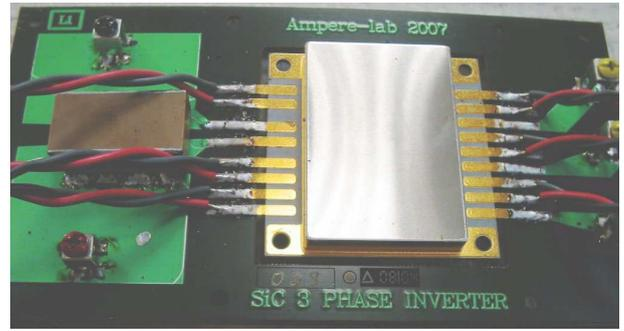
Fig. 13. Latest prototype. A 540VDC 15A three phase inverter operating at 200°C
